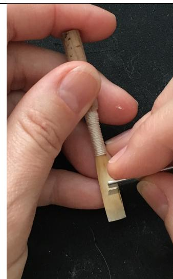
Because I prefer a smooth feeling reed, I turned the reed around and scraped backward from the heart into the back with a razor blade (this can also be done with a knife). This smoothed out any rough parts in the cane. Not only does it feel better in the mouth, but also I believe it helps to refine the sound of the reed.
