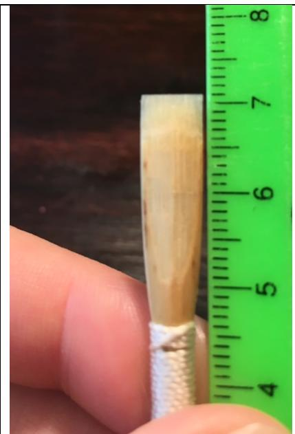
This is the finished reed. It is in tune, has a nice sound, is easy to articulate, and produces a large dynamic range. Notice where all the sections start and end. The total length is 71mm (which falls within the 69-71mm range). The heart falls between 61 and 66mm, and the back starts at 51mm.
