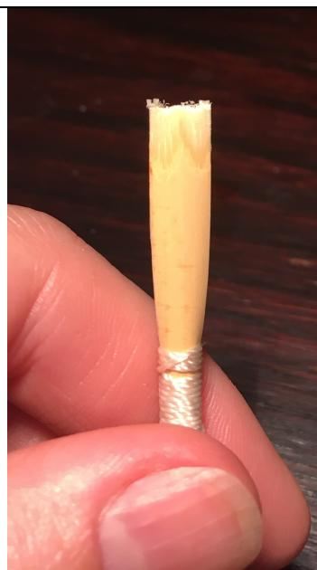
Scrape a “roughed-in” tip to form a tapered point. Start the scrape at 66mm. This is how I put my blanks away. Roughed-in tip, not clipped open.
