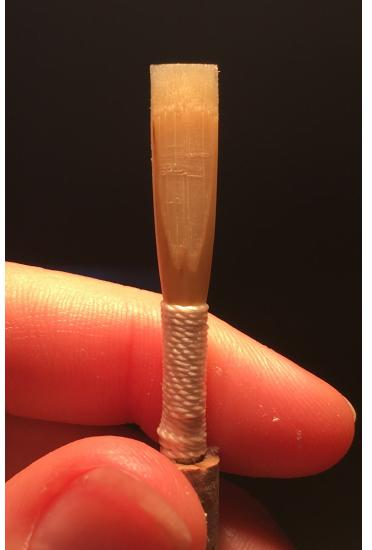
Notice the jaggedness of the scrape at the top of the back going into the heart. Later I will blend this by scraping from the heart into the back. I use a razor blade to smooth out the lines, but a knife is fine, too. Some people prefer to leave a notch here to define the back/heart.
