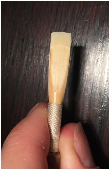
Another view of the back. You can really see the left rail on the heart here – this is a good width to leave the rails (about a  $\frac{1}{2}$ mm). Thinner than this and you lose stability and structure, thicker and the reed won't vibrate well.
