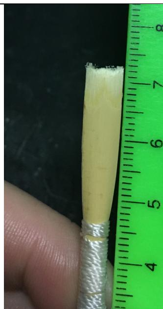
**Day 1:** The blank should measure 72-73mm from the bottom of the staple.
